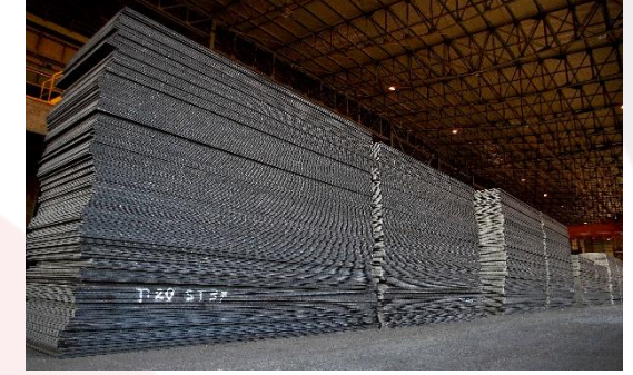
Cooperation in the production of Sheets (API 5L X60 MS sour service) of the national and strategic project of Goreh-Jask pipeline for the first time in Iran.
